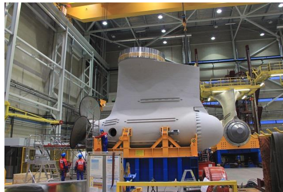
Factory Acceptance Tests of First Arc7 – 15 MW - Azipod (Dec. 2014)
